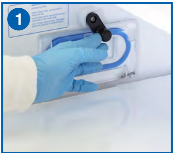
To use the Transfer Tunnel: open the hinged door in the Hypoxystation.
