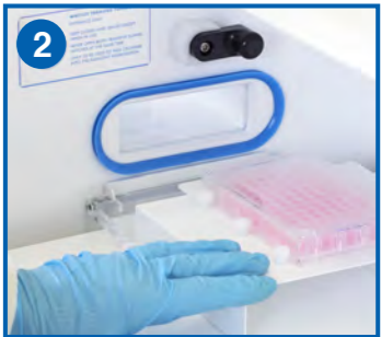
Place the cellware to be transferred on a holder in the Hypoxystation.
