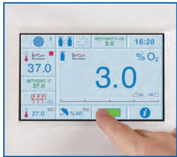
Intuitive operational software accessed via a full colour touch screen interface
